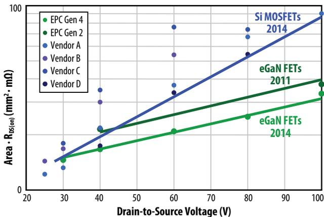
Figure 1: Specific on-resistance vs. blocking voltage capability for silicon MOSFETs and eGaN FETs.
