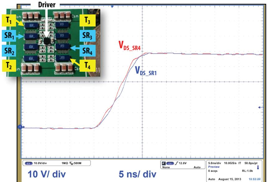
Figure 10: Four parallel GaN half bridge layouts and switching node waveforms with a single high frequency power loop (a) and four distributed high frequency power loops (b) ( $V_{IN} = 48$  V,  $V_{OUT} = 12$  V,  $I_{OUT} = 30$  A,  $f_{sw} = 300$  kHz, GaN transistors T/SR: EPC2001).
