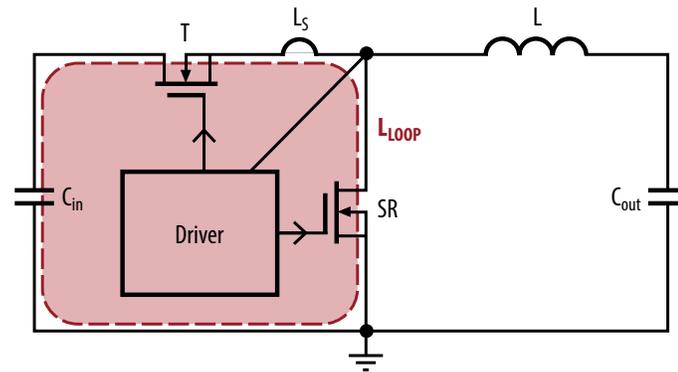
Figure 3: Synchronous buck converter with parasitic inductances.
