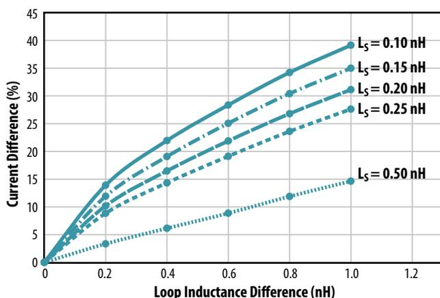
Figure 8: Impact of high frequency loop inductance imbalance on device dynamic current sharing for a  $V_{IN} = 48$  V,  $I_{OUT} = 25$  A, single phase GaN based buck converter with two half bridges operating in parallel for various common source inductances (GaN transistors: EPC 2001).
