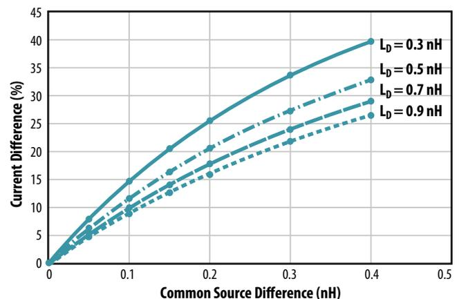
Figure 9: Impact of common source inductance imbalance on device dynamic current sharing for a  $V_{IN} = 48$  V,  $I_{OUT} = 25$  A, single phase GaN based buck converter with two half bridges operating in parallel for various high frequency loop inductances (GaN transistors: EPC 2001).
