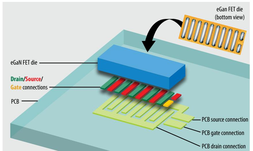
Figure 6: Exploded view of eGaN FET Land Grid Array package (LGA).
