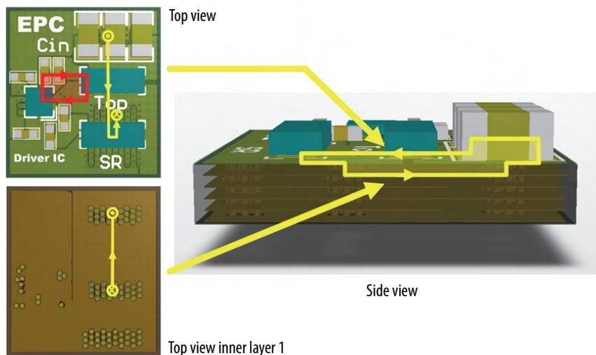
Figure 7: Optimal power loop with eGaN FETs top view, top view of inner layer 1, and side view.
