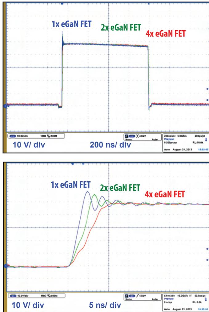
Figure 13: (a) Switching node waveforms with 1, 2 and 4 parallel GaN half bridges (b) zoomed view ( $V_{IN} = 48\text{ V}$ ,  $V_{OUT} = 12\text{ V}$ ,  $I_{OUT} = 30\text{ A}/\text{number of GaN FETs}$ ,  $f_{sw} = 300\text{ kHz}$ , GaN FET T/SR: 100 V EPC2001).
