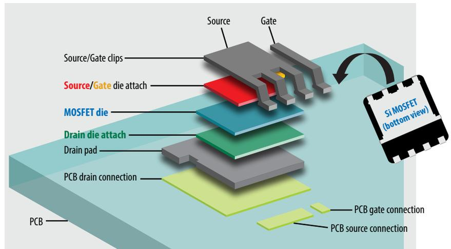
Figure 5: Exploded view of Si MOSFET Loss Free Package (LFPACK).
