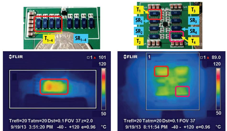
Figure 11: Thermal measurements of parallel GaN half bridge layouts with a single high frequency power loop (a) and four distributed high frequency power loops (b). ( $V_{IN} = 48\text{ V}$ ,  $V_{OUT} = 12\text{ V}$ ,  $I_{OUT} = 30\text{ A}$ ,  $f_{sw} = 300\text{ kHz}$ ,  $L = 3.3\text{ }\mu\text{H}$ , GaN transistors T/SR: 100 V EPC2001, fan speed: 200 LFM).
