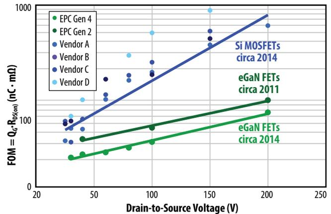
Figure 2: Gate charge FOM comparison of eGaN FETs and state-of-the-art Si MOSFETs for drain-to-source voltages at half of their rated voltage and a drain-to-source current of 20 A.
