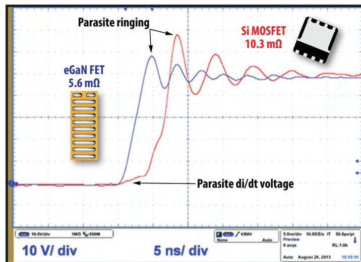
Figure 4: Switching node waveforms of eGaN FET and MOSFET designs ( $V_{IN} = 48 V$ ,  $I_{OUT} = 10 A$ ,  $f_{sw} = 300 kHz$ , GaN transistors: EPC2001 MOSFETs: BSZ123N08NS3G).
