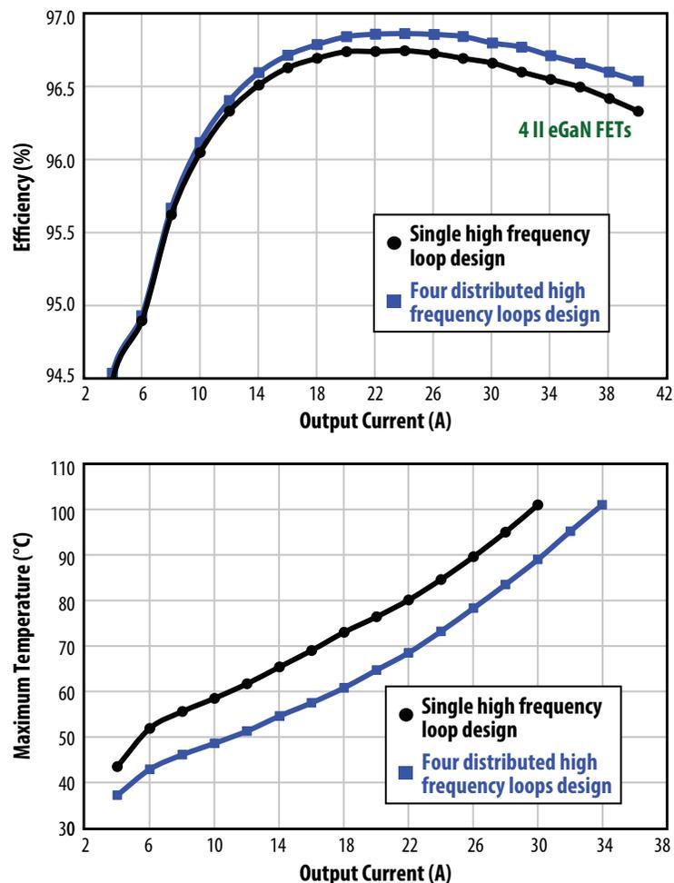
Figure 12: Efficiency (a) and thermal comparison (b) for conventional and proposed parallel GaN half bridge designs ( $V_{IN} = 48\text{ V}$ ,  $V_{OUT} = 12\text{ V}$ ,  $f_{sw} = 300\text{ kHz}$ ,  $L = 3.3\text{ }\mu\text{H}$ , GaN transistors T/SR: EPC2001).
